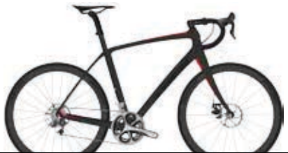
DOMANE SLR 9 DISC Matte Dnister Black/Viper Red RAHMEN 600 Series OCLV Carbon, Front and Adjustable Rear IsoSpeed GABEL Domane Disc-Gabel aus Vollcarbon SCHALTWERK Shimano Dura-Ace Di2 KURBELGARNITUR Shimano Dura-Ace LAUFRÄDER Bontrager Aeolus 3 Tubeless Ready D3 Disc
