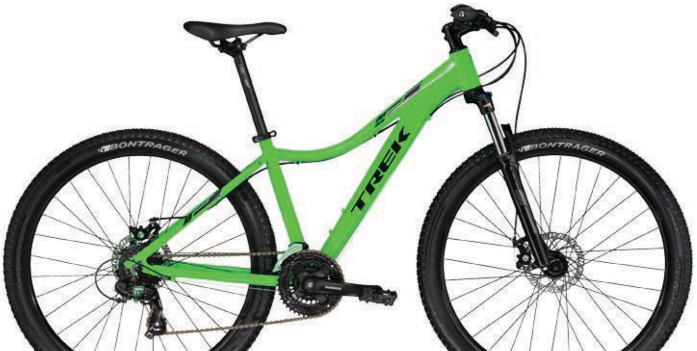
SKYE S WSD Green-light RAHMEN WSD Alpha Silver Aluminium FEDERUNG SR Suntour XCT, 100 mm Federweg (13,5: 80 mm Federweg) SCHALTWERK Shimano Tourney TY300 KURBELGARNITUR Shimano Tourney TY501 LAUFRÄDER Formula alloy hubs; Bontrager Connection rims
