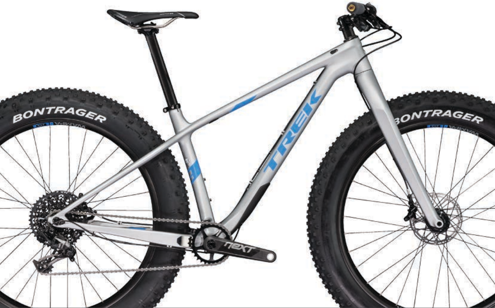
FARLEY 9.8 Matte Quick Silver RAHMEN OCLV Mountain Carbon SCHALTWERK SRAM X01, Roller Bearing Clutch KURBELGARNITUR Race Face Next LAUFRÄDER Trek Wampa Carbon 80 SL, Tubeless Ready, 150 x 15 mm vorne, 197 x 12 mm hinten
